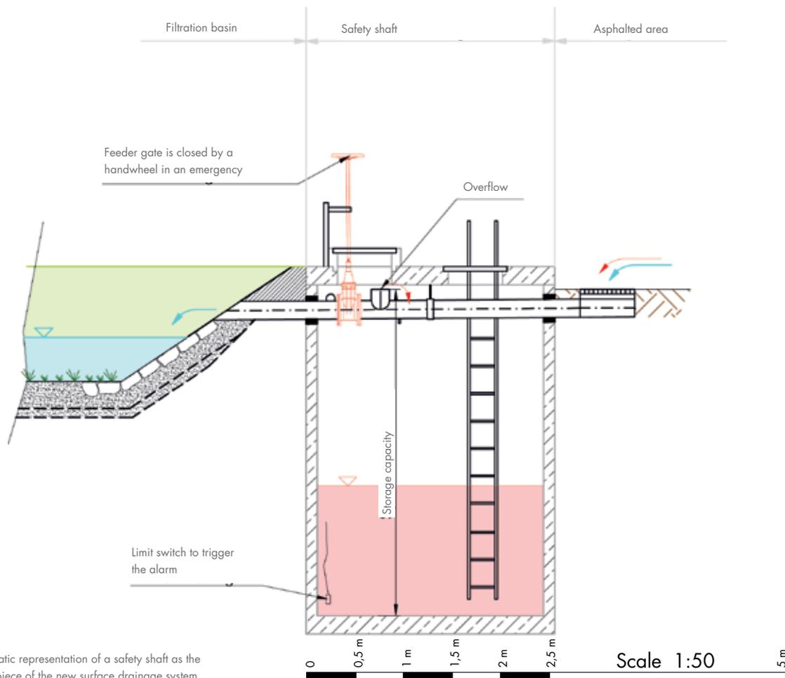
Schematic representation of a safety shaft as the centrepiece of the new surface drainage system
