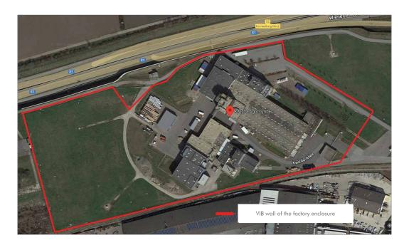
Between June and December 2014 the factory was enclosed with a VIB-wall approximately 815m long as a measure to ensure the long-term protection of the groundwater body "Korneuburger Bucht".
